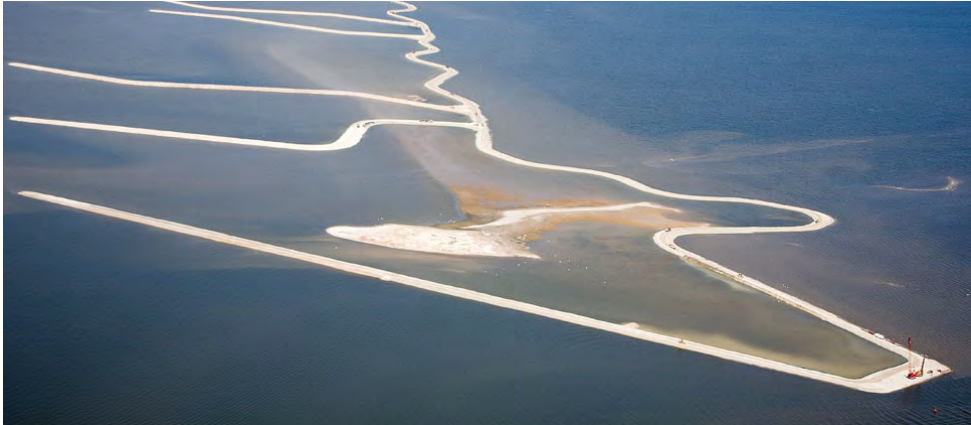
Aerial view of the Cat Island project, including the stone seawall used as a base for stability. Photo by the Army Corps of Engineers
