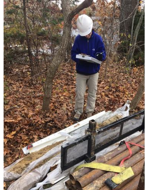
Dr. Erban logging sediment core samples during well installations for the project in November 2019.
