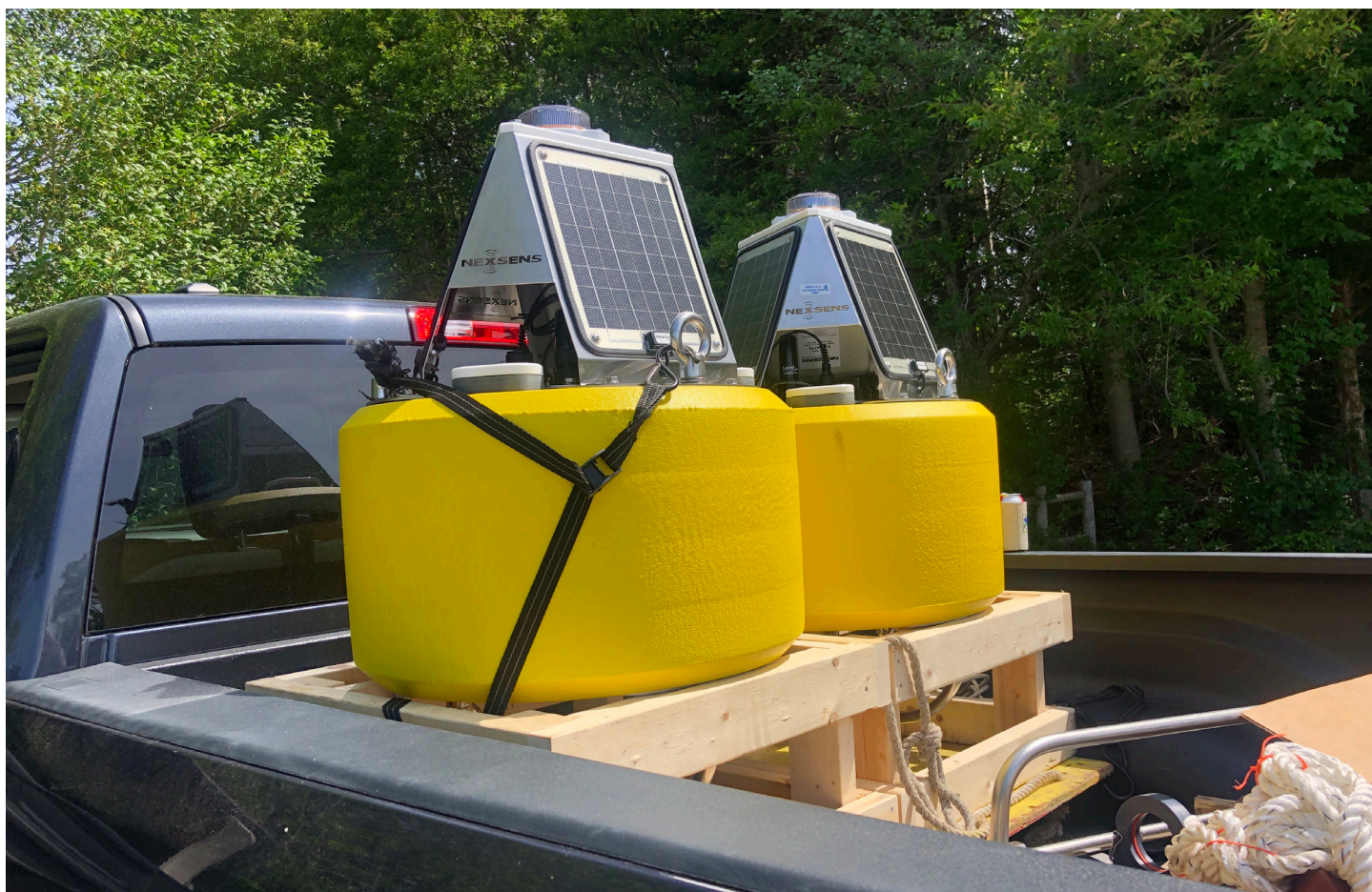
Pictured are the two EPA sensor buoys being used to collect data on HABs. One buoy was placed in Shubael Pond and the other in Hamblin Pond.
