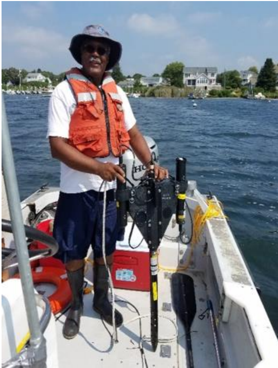
Darryl Keith with the in-water HyperSAS profiling radiometer system which measures the spectrum of the underwater light field. This system will provide in-water validation of remote sensing algorithms to map seagrass density and estimate phytoplankton and cyanobacteria concentrations derived from satellites, aircraft, and UAV data
