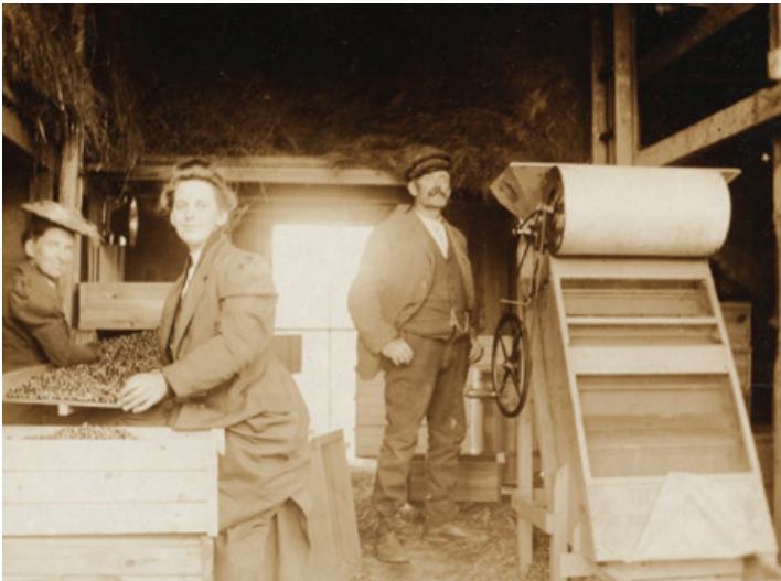
A screening machine separated spoiled cranberries from good ones through a bouncing process. Skilled workers were still required to handpick cranberries before being shipped.
